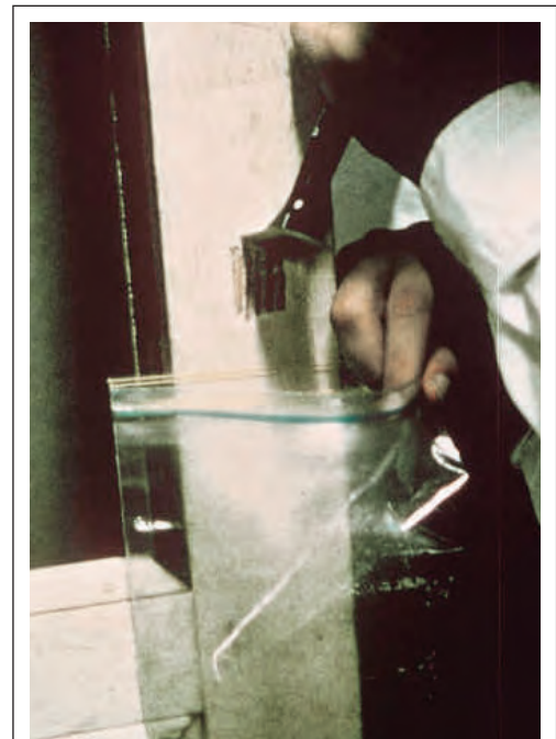
FIGURE 7.5 Removing paint-chip sample.
