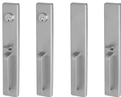
512TP 512NL 512DT 512TP-BE Escutcheon: 16" x 2 3/4" Grip: 6 1/4" C-C Projection: 2 11/16" Brass For keyed functions, see page 14 for cylinder requirements.
